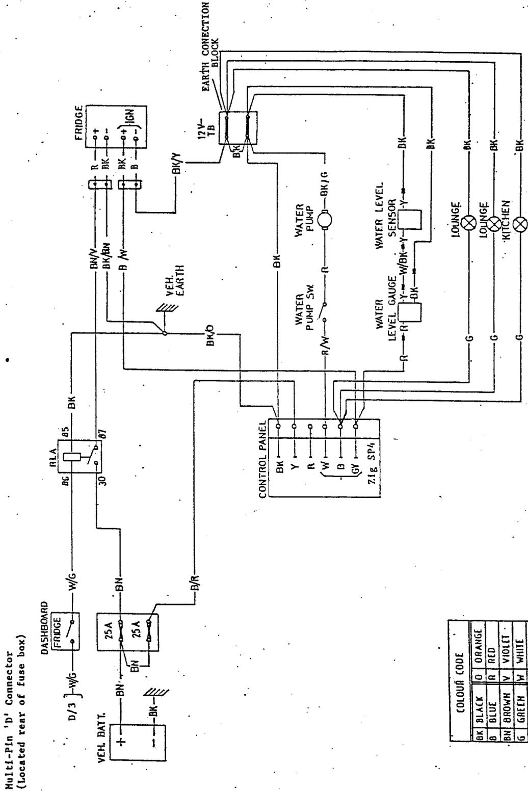
T4 VISION 12V WIRING DIAGRAM
