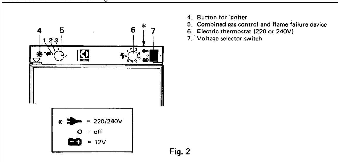
The bottled gas equipment includes a Piezo crystal lighting device which creates a spark over the burner when the button (4) is pushed in fully. No batteries or flints are required to operate this lighter.
