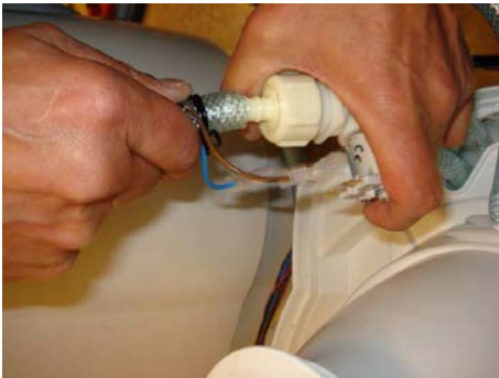
Push tube onto valve
