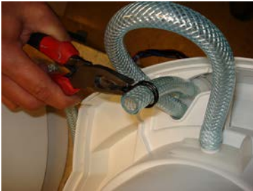
Slide hose clamp over tube
