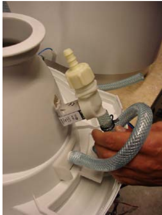
Push new valve in tube, arrow should be in direction of water flow
