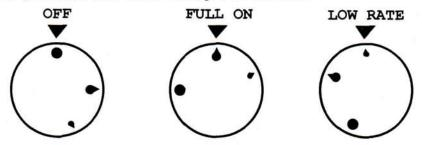
To light the burner,depress and turn the knob anti-clockwise to the full rate position. Hold the knob depressed and apply a light to the burner. It is necessary to hold the knob depressed for approximately 15 seconds after the burner has lit to allow the probe to reach temperature. Should the flame go out when the knob is released, the procedure should be repeated holding the knob depressed for slightly longer. If required the knob can be turned further anti-clockwise to the simmer position.
