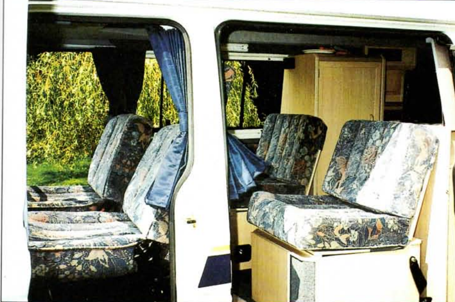
Four seats at Vision's front will convert to twin single beds or inward facing settees. Upholstery looks (and is) luxurious.
