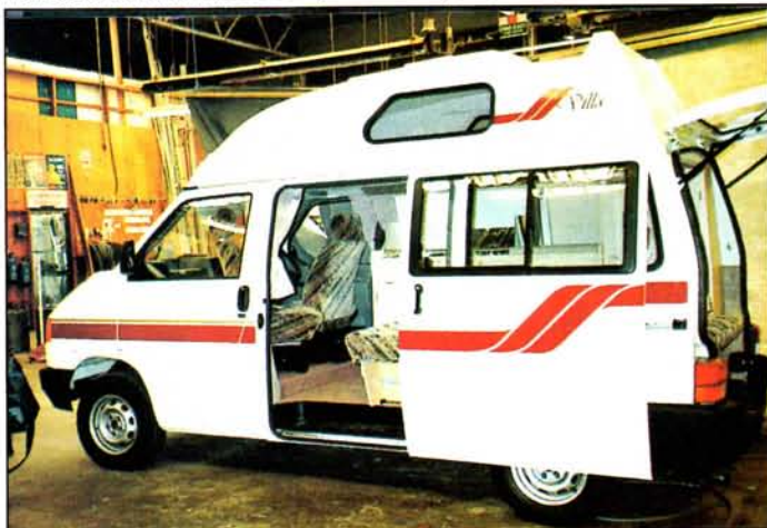
Villa in workshop. Stowage area which takes the place of the rear engine can just be seen. High roof incorporates a roof rack.
