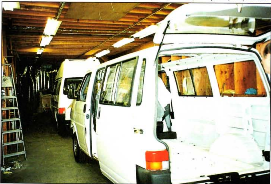
In Holdsworth's body shop. Roof cut-out on van nearest camera has yet to be strengthened to conform to VW's exacting standards.
