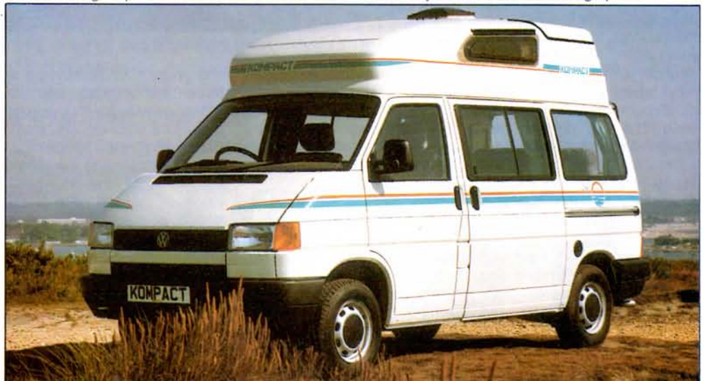
Two-berth Autohomes Kompact has a lower roof-line with a built-in 'top-box' and ladder at the back
