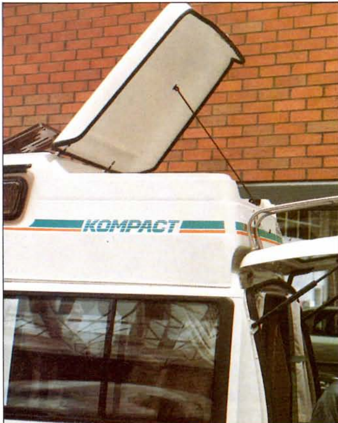
Kompact's rear luggage compartment lid is moulded into the roof-line
