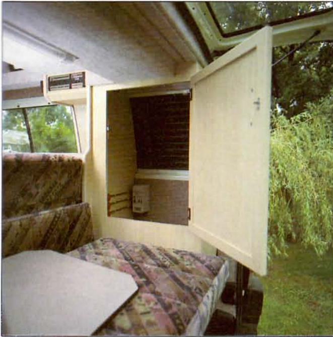
Villa's wardrobe is in the traditional VW position behind the settee; visible are the mains RCD unit and isolator taps for gas appliances
