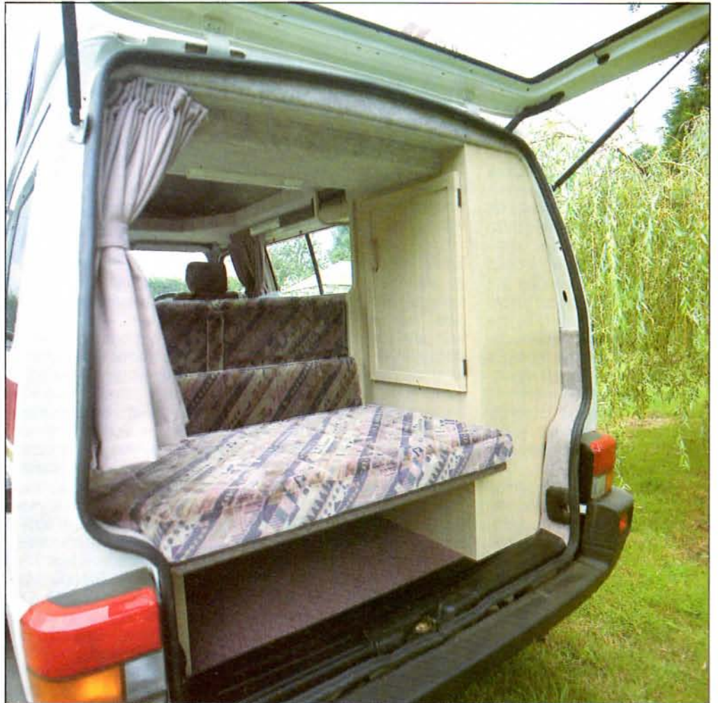
Rear storage shelf and 'boot' area, where items can be kept out of sight. Tailgate now extends down to rear bumper height
