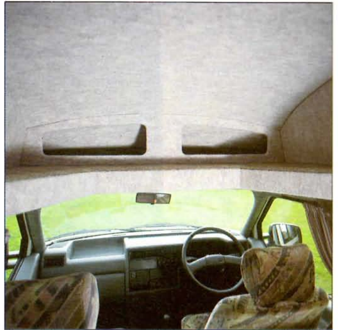
Open lockers provide additional storage over the cab, where the roof-cut-out tapers inwards
