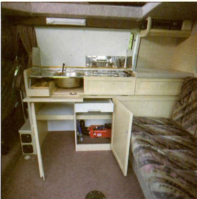
Stainless steel appliances are beneath kitchen worktops; left-hand cupboard takes a portable toilet; Propex heater in right-hand cupboard will be properly boxed in – one of Villa's optional extras
