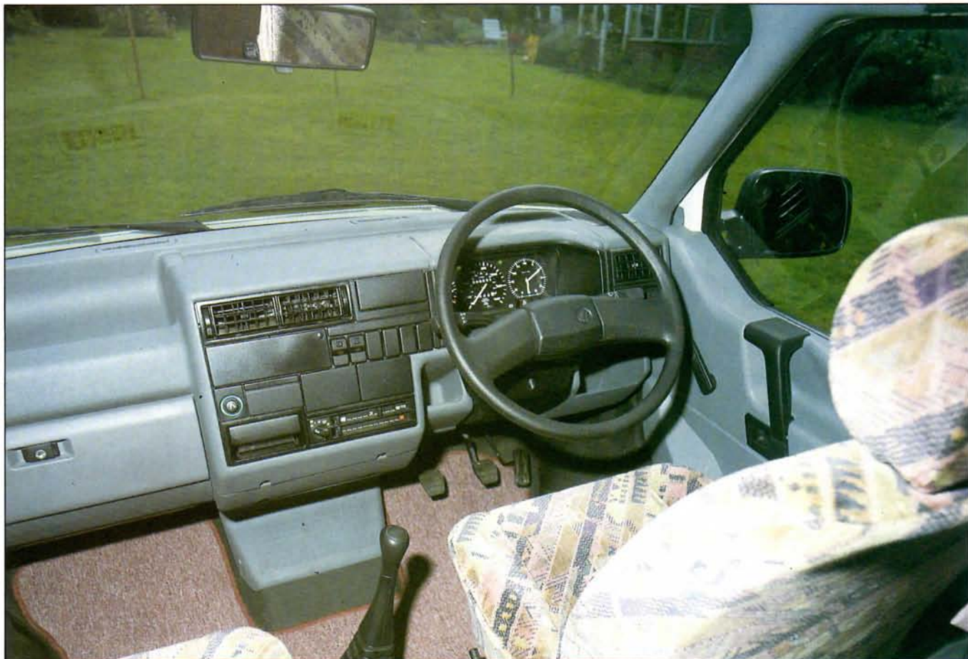
Transporter Kombi's cab seats, including headrests, are upholstered to match soft furnishings; dashboard and facia are finished in grey/black vinyl to reduce glare; all major and minor controls fall easily to hand
