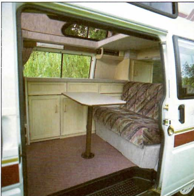
Interior layout looks similar to earlier Villas; Electrolux fridge has been replaced by a top-loading 12v/240v/gas unit, allowing more storage in kitchen cupboards
