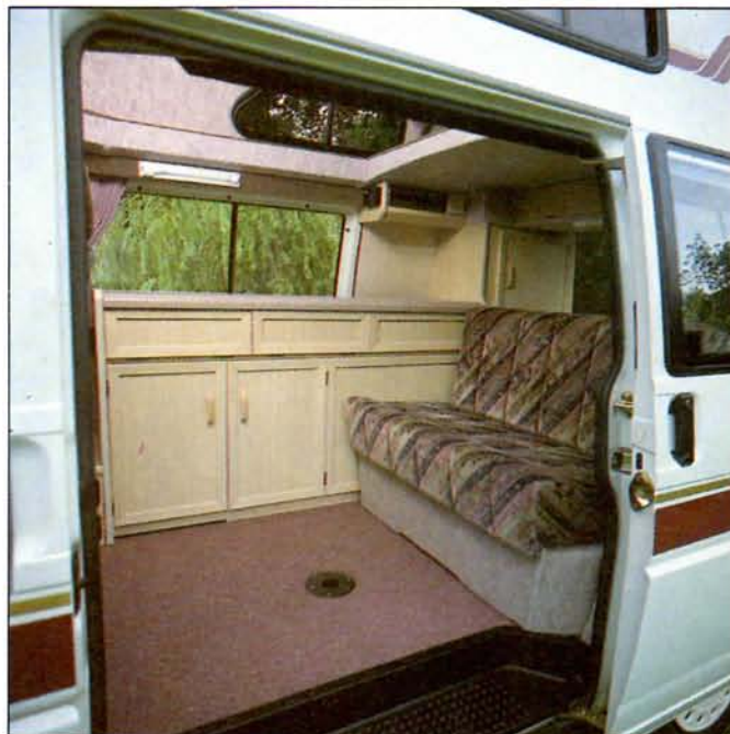
Transverse settee is fitted with lap belts and is now built on a metal-framed base; anchorage points and frame have been crash-tested
