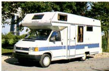
Auto Trail Cree • No. of berths: 4 • Length: 6.13m • Width: 2.20m • Height: 2.77m
