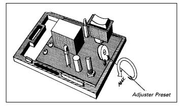
The preset is not a linear control and most of the adjustment is toward the anticlockwise endstop.
