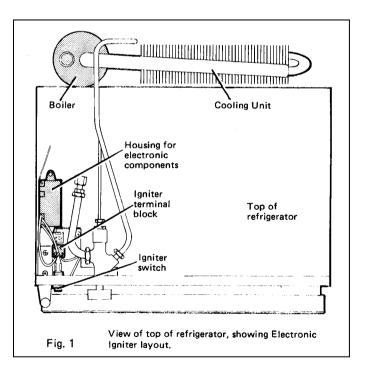
If the burner does not re-ignite within 30 to 60 seconds, the flame failure valve will close and automatically shut off the flow of gas to the burner. If this happens, sparking will continue to take place and the neon light in the switch will flash continuously to alert the user that something is wrong, or that the gas bottle is empty and needs replacing.
