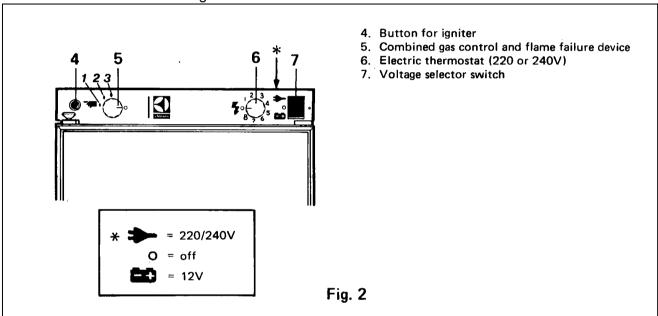
The bottled gas equipment includes a Piezo crystal lighting device which creates a spark over the burner when the button (4) is pushed in fully. No batteries or flints are required to operate this lighter. Before starting the refrigerator, always check that the alternative method of operation is off as the refrigerator should not be operated by both means at the same time. If the caravan is to be stationary for a period, check that the refrigerator is level.
