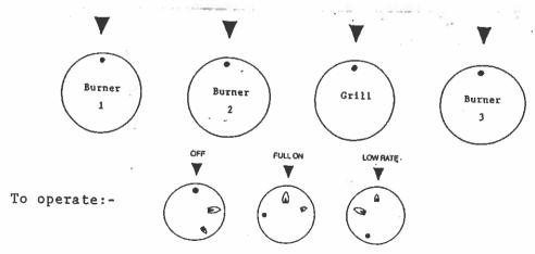
Never allow a full flame to burn without a utensil over the burner as this is wasteful and it may also result in heat damage to the underside of the cooker lid or the headlining immediately above the cooker. Care should also be exercised in operating gas taps, because of the restricted space between the chrome windshield and the taps, this area can become extremely hot when the burners are alight.
