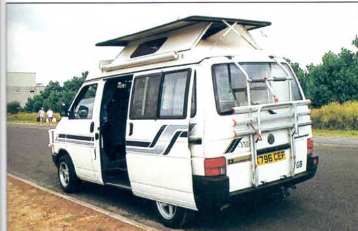
A push on the centre of the roof and the gas struts take up the hard work.
