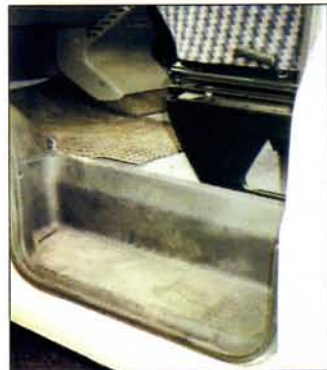
The large inset step is plastic-lined and the rubber mats keep the carpet clean.
