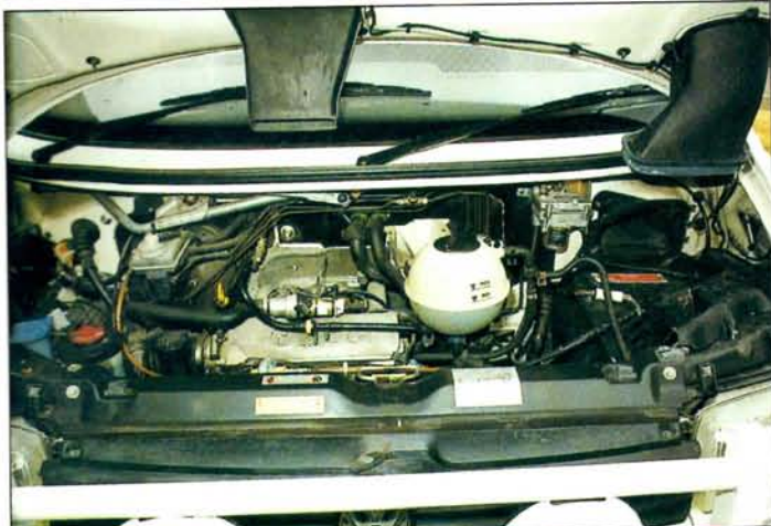
A 2.5-litre, 5-cylinder, fuel-injected petrol engine provides more than enough power.
