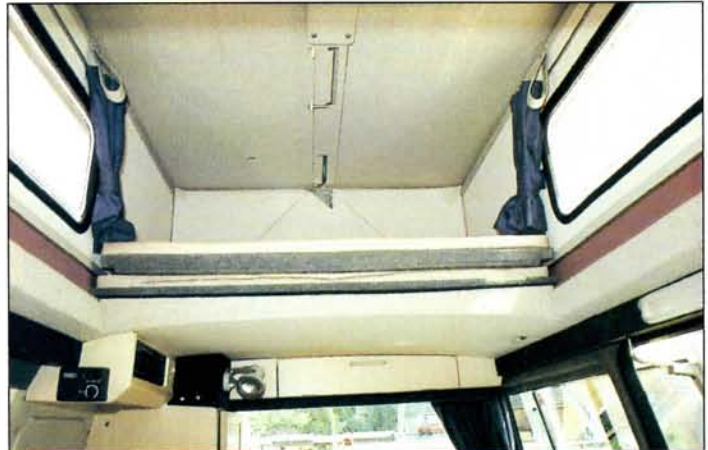
The clever design of the long bolt ensures the roof panel is eased and locked into place.
