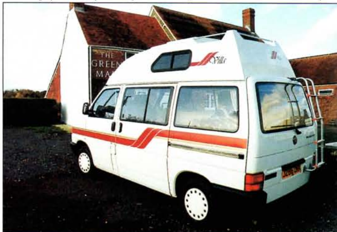
Roof rack, which is easily reached from the ladder on the tailgate, offers extra storage capacity.
