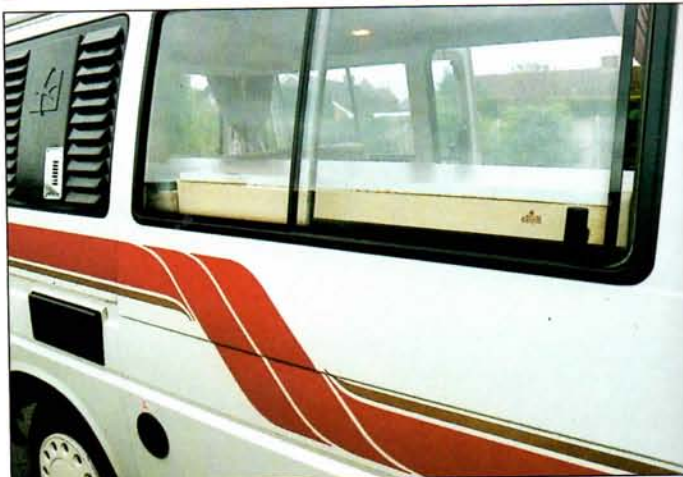
Holdsworth arrangement keeps the fridge flue well away from the offside opening window.
