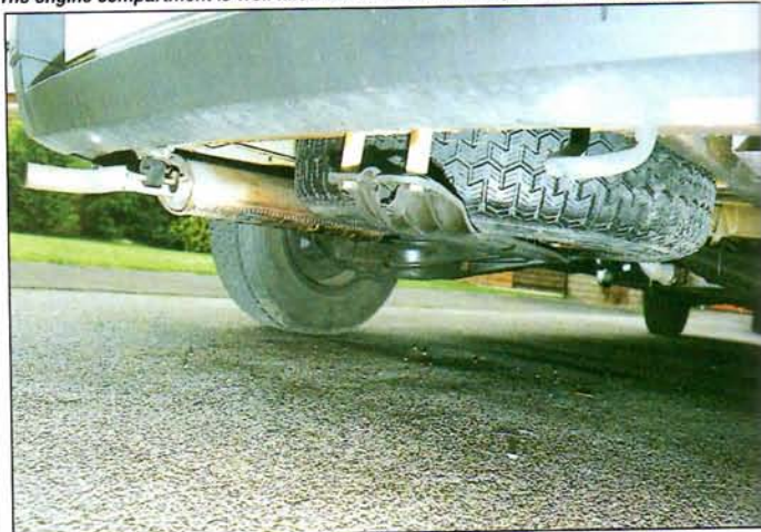
Spare wheel, in cradle forward of rear bumper, is released by turning two bolts with wheelbrace.
