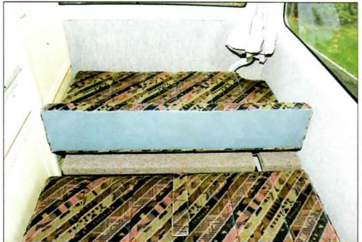
Hinged central section simplifies bed making and will be softer on production models.
