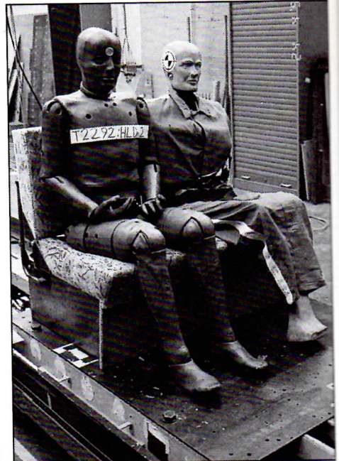
Adult dummies are strapped to the rear seat ready for their impact, involving a force of 20G.
